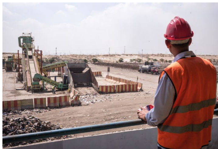
Worker looking over the plastic bag sorting, shredding, and compacting facility at the waste management operation at the Egyptian Company for Solid Waste Recycling © NSWMP/David Degner
