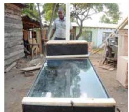
Direct Mode-Solar Sludge Drier
