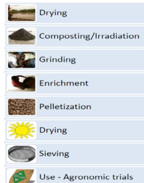
This study confirms that it is possible to produce excreta-based pellets in small and medium size enterprises with local machinery. Upcoming studies will include testing the pellets in a greenhouse to confirm their suitability for different soil types and crops. If successful, such application could help make faecal sludge reuse a clean and safe process for private entrepreneurs as well as farmers.
