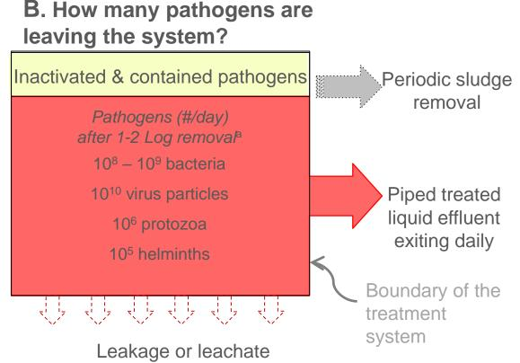
(A sealed septic tank would have no flow here)
