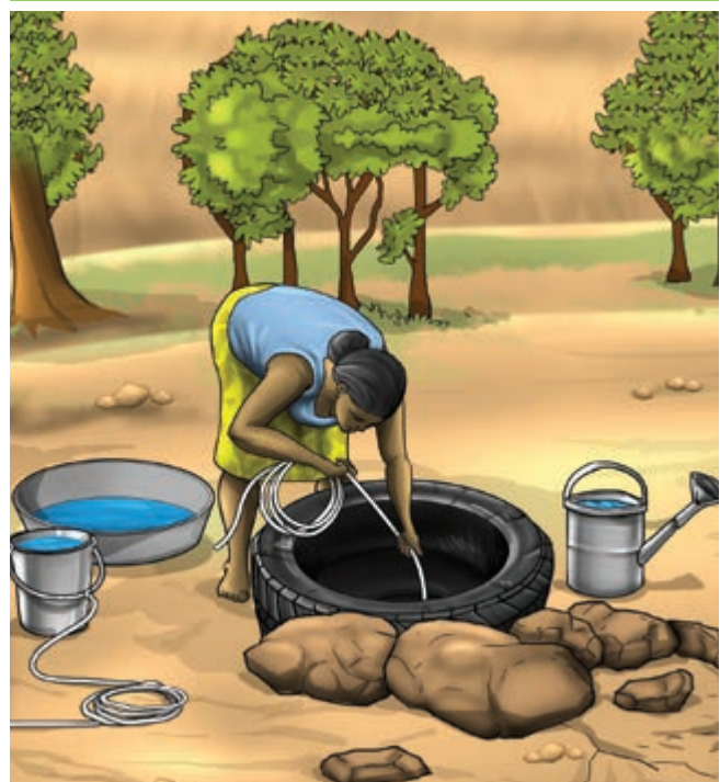
FIGURE 11. SIMPLE WELL STABILIZED WITH RUBBER TIRES CLOSE TO A POLLUTED STREAM. WATER IS FETCHED WITH A BUCKET AND ROPE.
