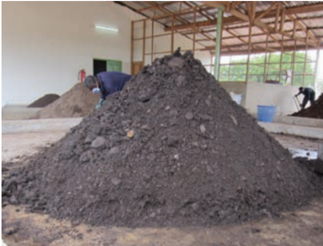
FIGURE 16. HEAP COMPOSTING OF DEWATERED FS.
