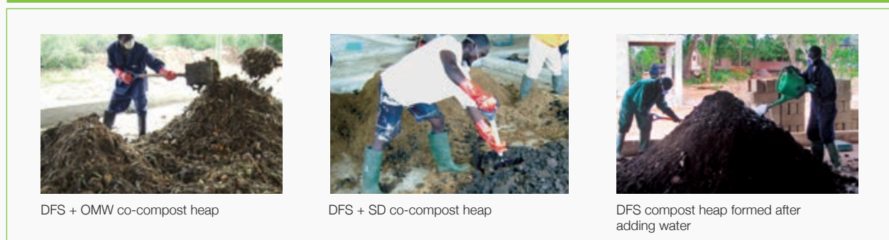
FIGURE 17. FORMATION OF THREE COMPOST HEAPS (ACCRA, GHANA).
